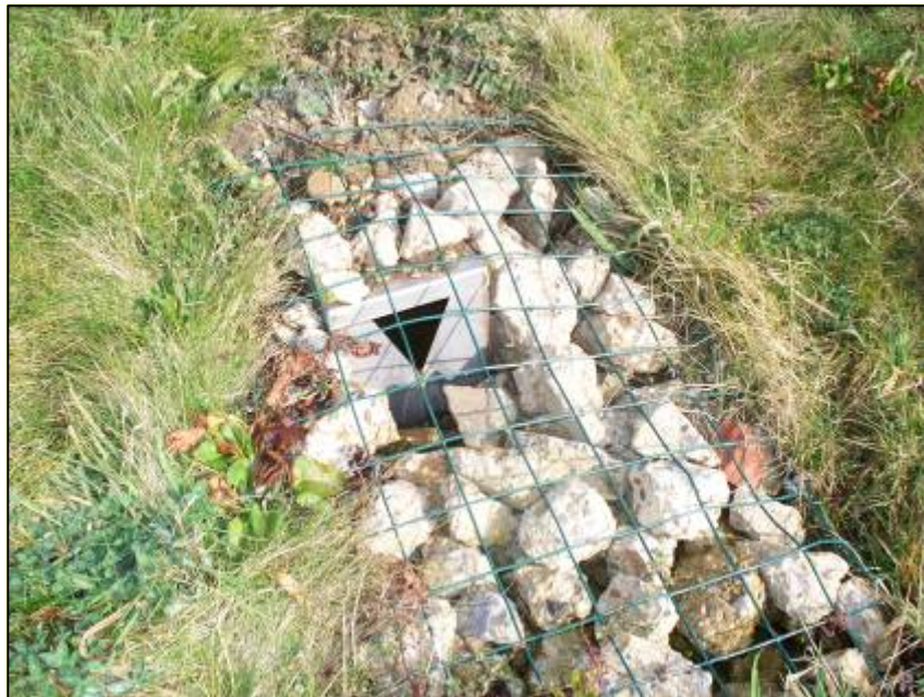
Figure 2.2: V-notch weir control structure at the Study Site
