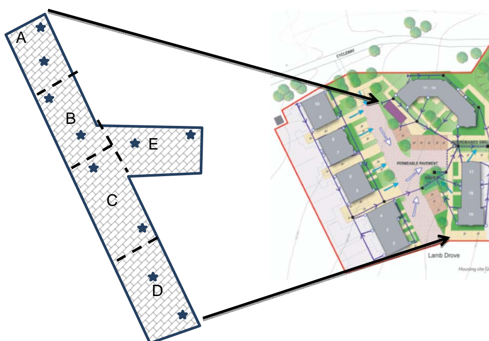
Figure 2.5: The infiltration measurement points on the permeable pavement
