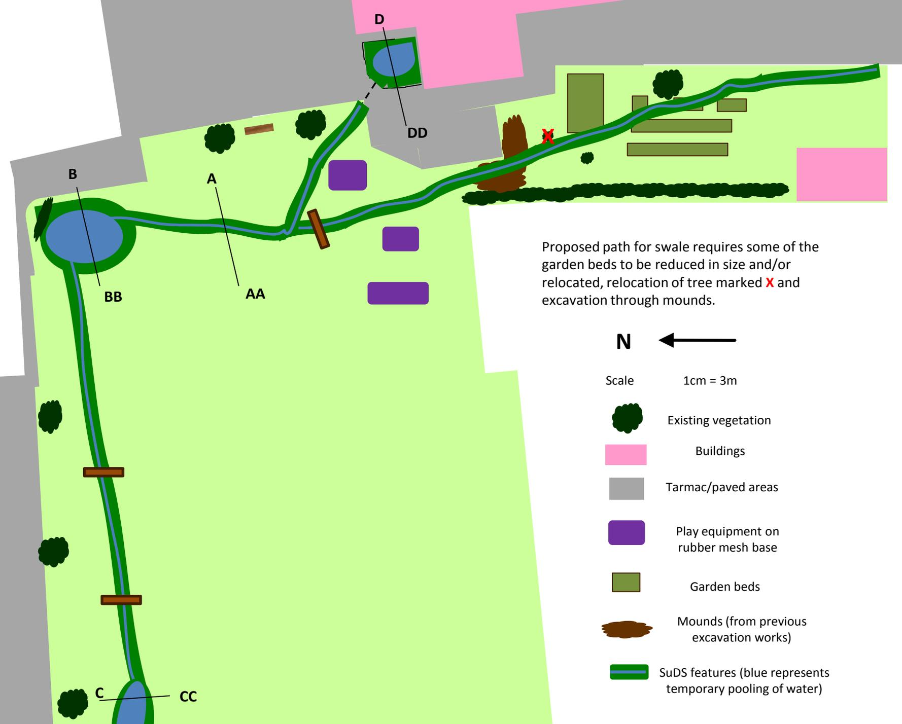
Proposed path for swale requires some of the garden beds to be reduced in size and/or relocated, relocation of tree marked X and excavation through mounds.
