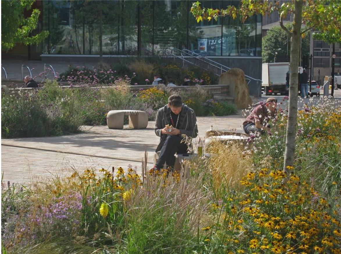
Linear source control Bio-swales gardens running along the highway, cycleway and receiving all hard paved surfaces with. (see below construction detail). The image shows the potential calming and mental restorative effects that this style of planting can provide. All planting provides SuDS benefits.
