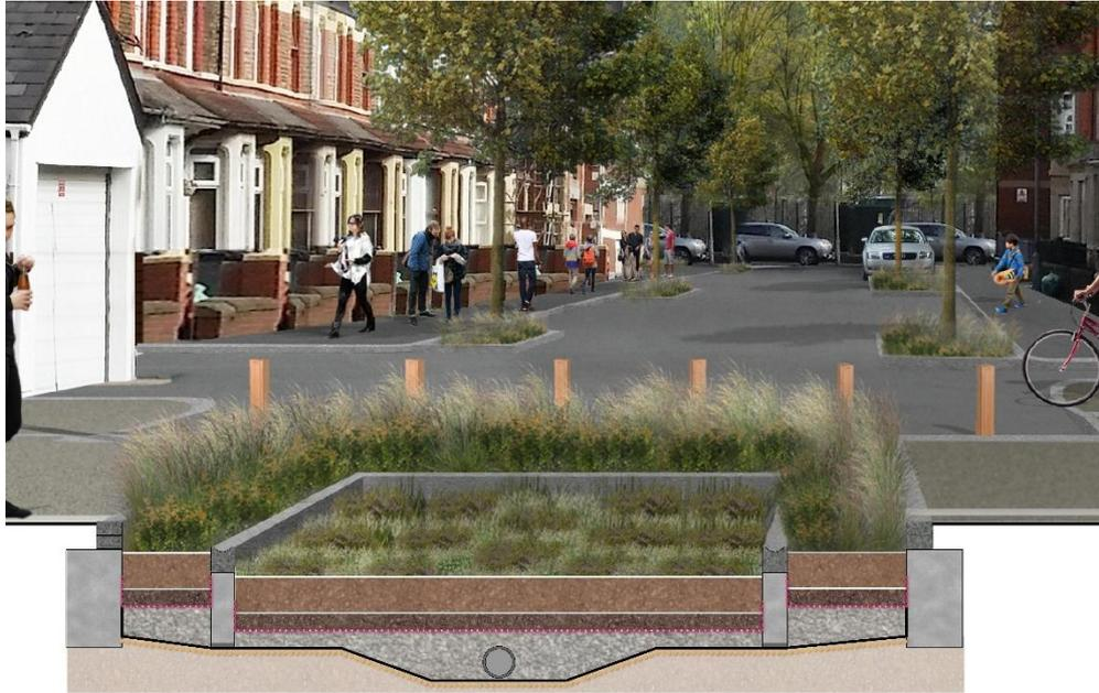
Figure 3 – Artistic impression of section through rain garden showing perforated pipe at the base
