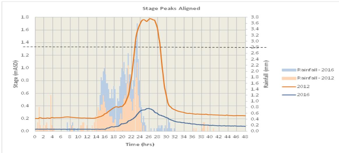
The graph shows the two peaks aligned in the 10 hours over the event and shows a very substantial reduction in peak level. The gauges were checked to ensure that there were no technical errors or problems and the 2012 data was compared with other events pre-construction. The November 2012 graph is a consistent level of response. The data for both events is reliable.
