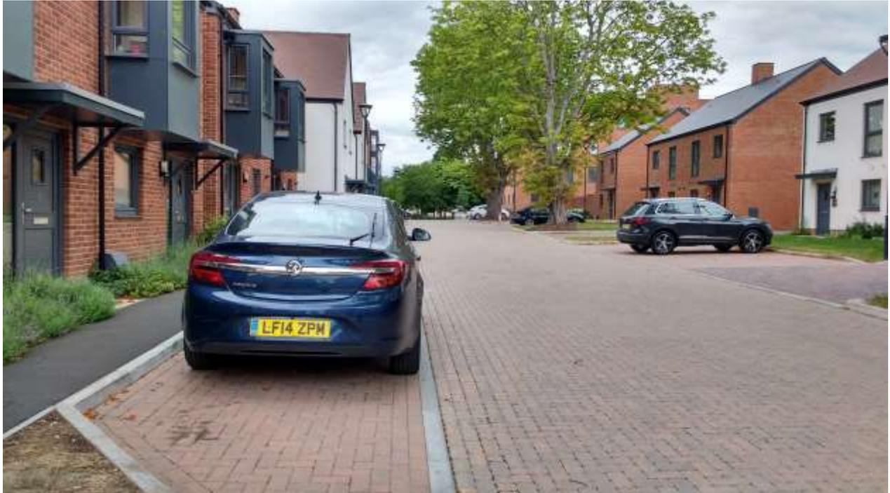
Fig 1: Permeable Paving within Parcels. Waterbutts on each house to the rear.
