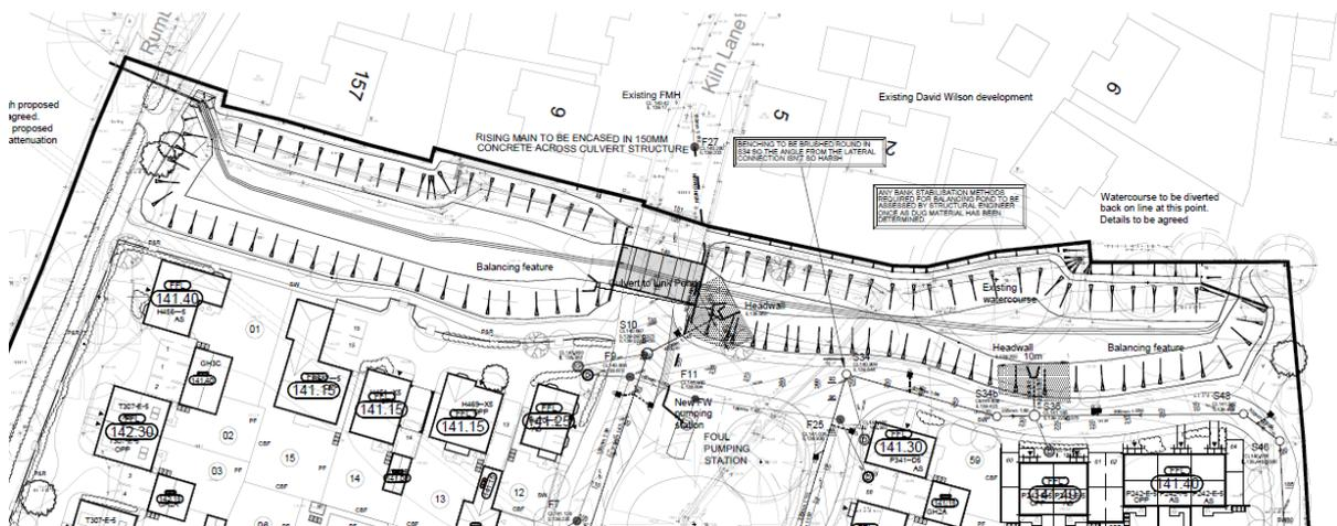
Fig 5: The resultant design showing the 2 connected swales with bridge providing access
