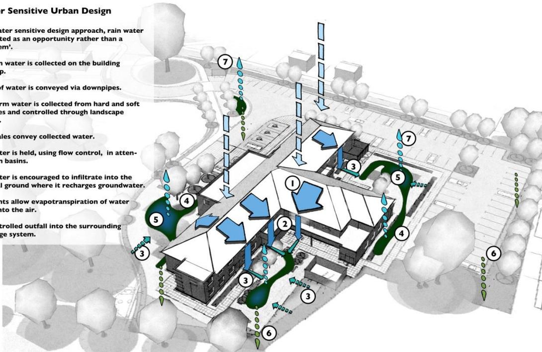
Figure 3 Schematic showing concept of water sensitive urban design for Alchester Health Centre
