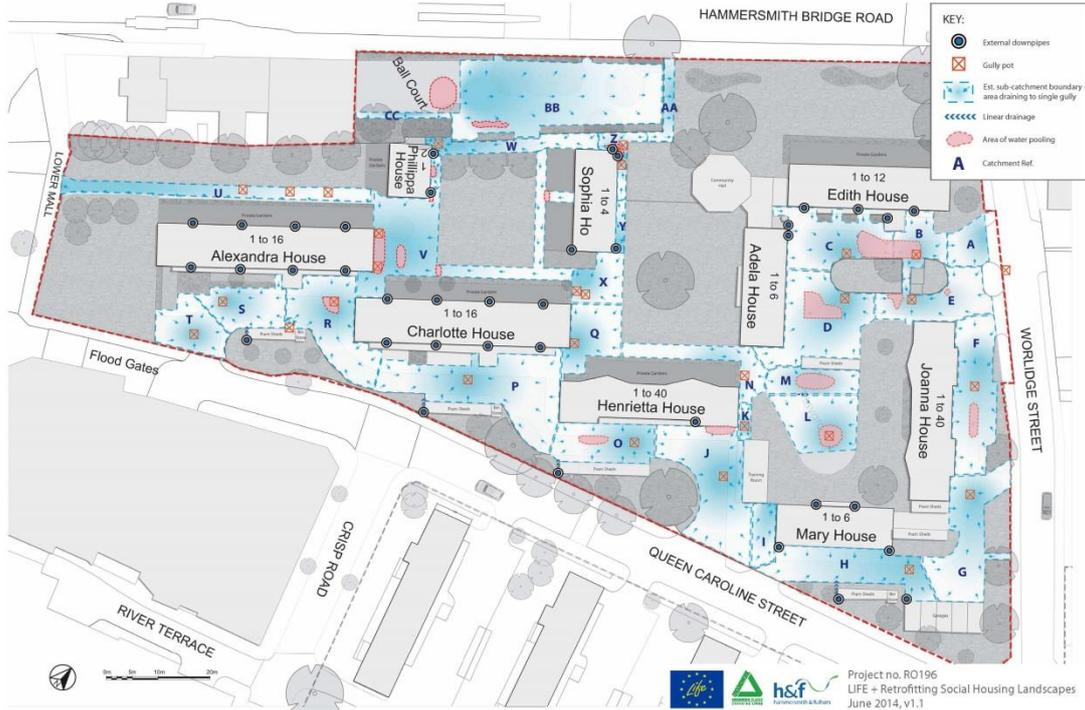
Fig 2 Queen Caroline Site Plans - drainage and flow analysis
