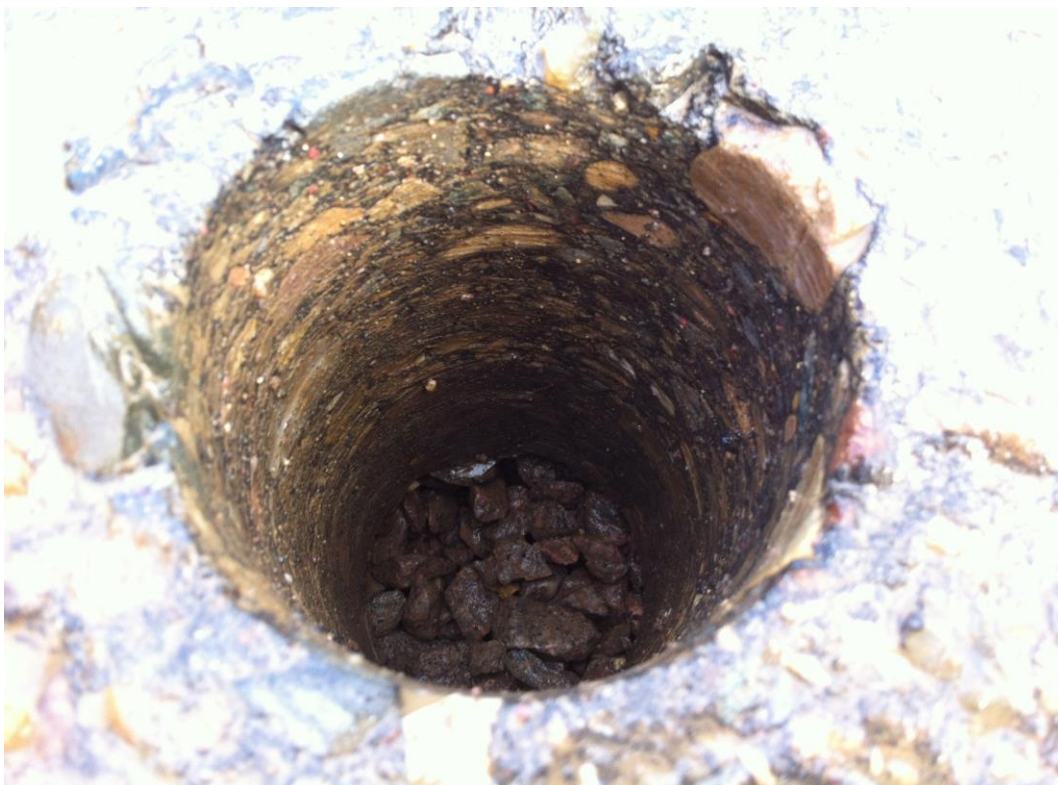
Fig 5: DBM core showing permeable sub-base beneath
