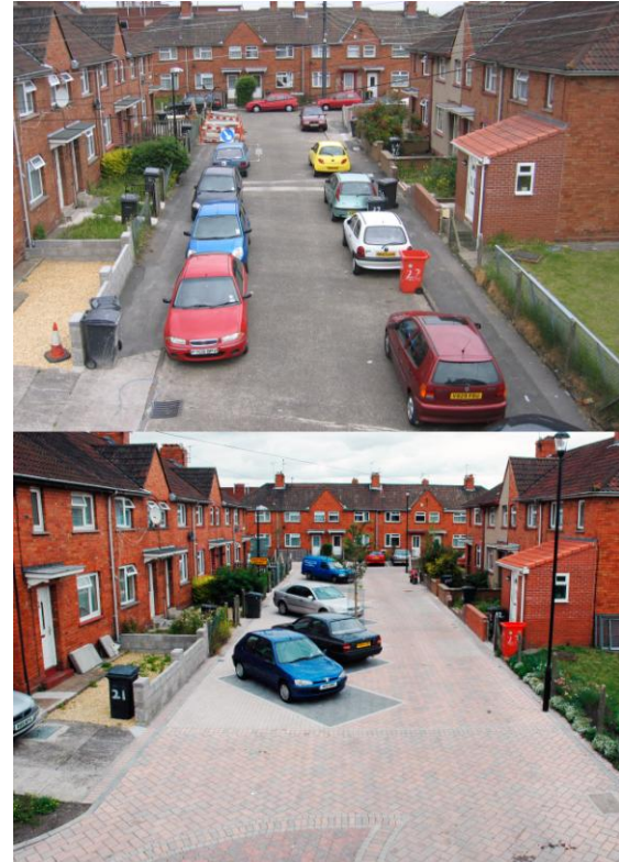
Figure 7 The Dings, Bristol where permeable pavement was retrofitted during the creation of the 'Homezones' area (courtesy of Sustrans).
