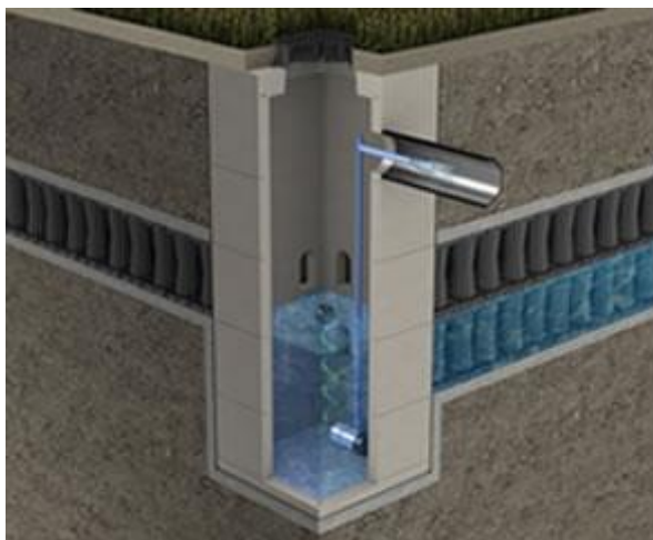
Figure 5 Subsurface attenuation installation and access chambers
