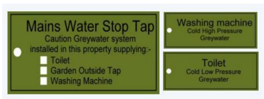
Figure 4-8: Examples of labels for use at stop valve and other key connection points (extract from WRAS Information & Guidance Note No. 9-02-05)
