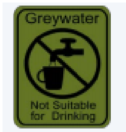
Figure 4-7: Examples of labels for storage cisterns and point of use appliances e.g. washing machines, WCs, outside taps (extract from WRAS Information & Guidance Note No. 9-02-05)
