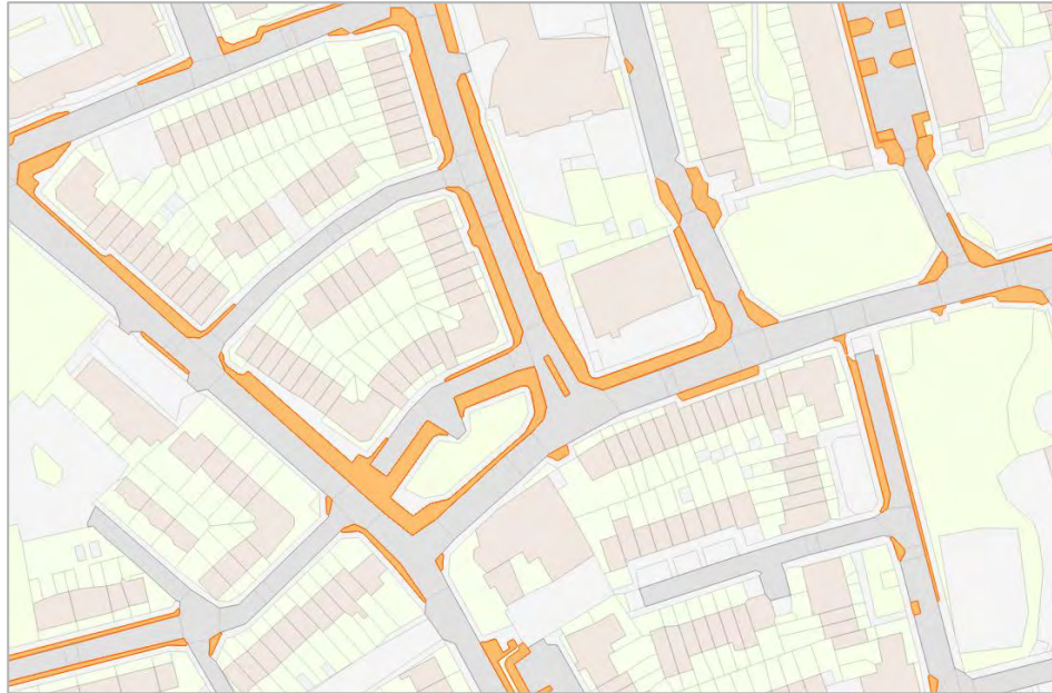
Figure 12 – Streetscape Bioretention, Example of SuDS Feature Delineation
