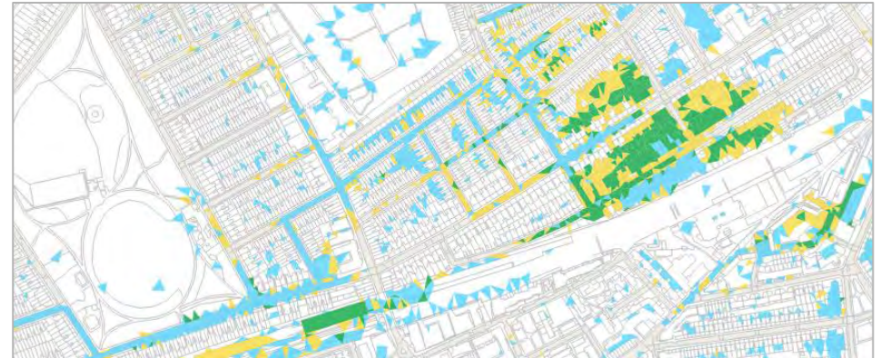
Figure 48 – All Streetscape SuDS 25% Realisation Level, Flood Mitigation Potential Around Kilburn Area
